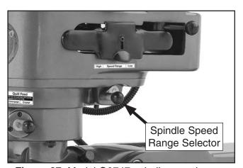
**Figure 27.** Model G0747 spindle speed range selector in the forward (high) position.
